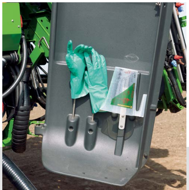
✔ A holder for gloves and a measuring jug are provided in the inner panel of the operator station cover
